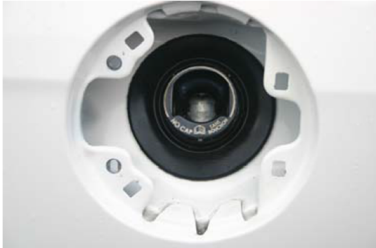
Fig. 1 – Flange Gasket installed after plastic pocket & stock door removal
